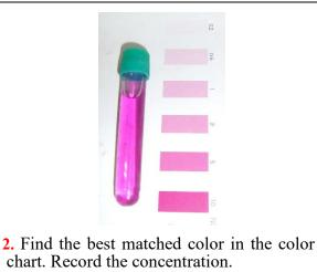
Fill a tube with sample water. Cap the tube and shake vigorously until the reagent completely dissolves. Wait 5 minutes.
